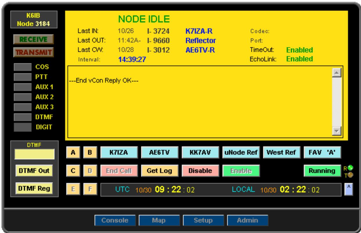
The IRLPVCON package was created to provide a complete real-time visual admin console for an IRLP node. It provides all of the monitoring and control functions necessary to operate an IRLP / EchoIRLP node using a JavaScript Enabled Web Browser. It also includes a real-time status monitor (IRLPvMON) and connection map monitor (IRLPvMAP).
