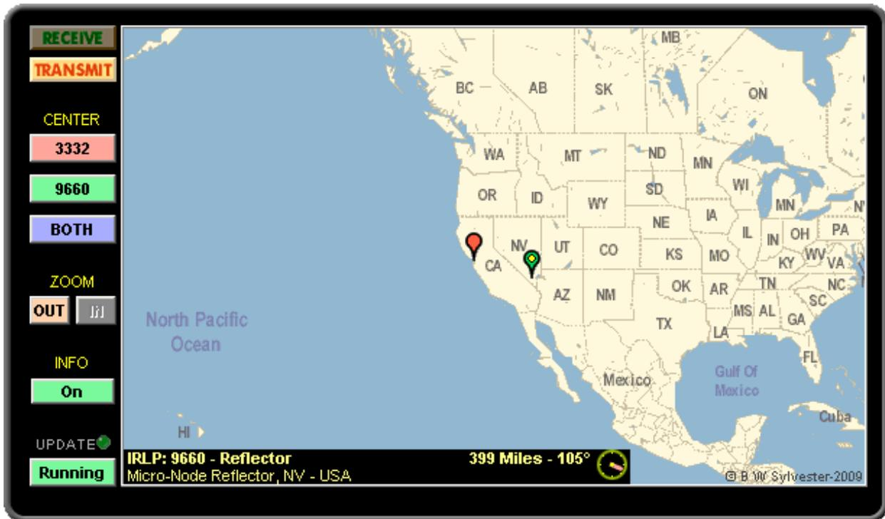
The IRLPvMAP Monitor Screen is a real-time map display that shows your node's location and the location of any IRLP node that is connected to it. To work It requires the Latitude and Longitude information be set using the Setup Screen.
