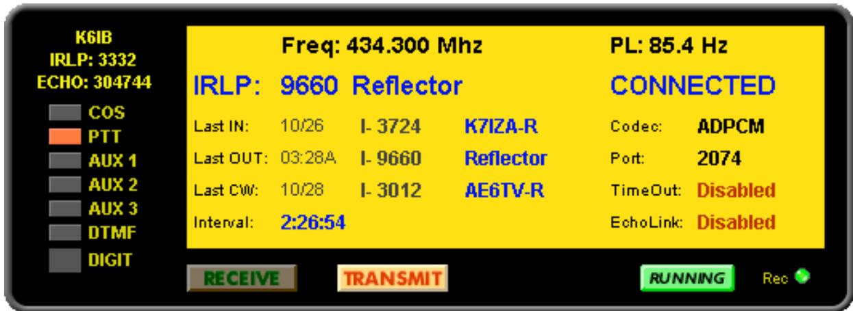
The IRLPvMON Monitor Screen is a display that shows the real-time status of the node. It is a Monitor Only and has No Control Capability.
